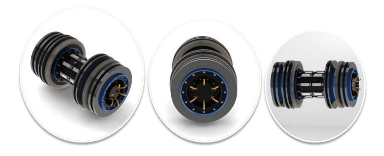
Designed to remove and avoid build-up of sand, wax, scale, black powder, and other debris in front of the scraper. Percentage of propelling fluid is allowed to pass through the scraper from the rear forward. This flow will pass ahead of the scraper creating turbulent flow and keeping the debris flushed or suspended ahead of the scraper preventing build-up and blockage which could cause the scraper to get stuck.
