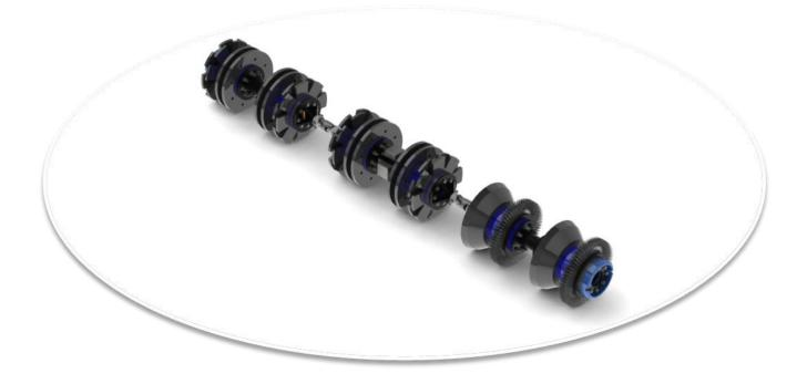
Can be modified to run in dual-diameter and multi-diameter pipelines as well as through features such as Wyes, Unbarred Tees, and Check Valves. Pigs are suitable for safe backloading into subsea PLRs as well as onshore Pig Launchers. Further, add-ons can be incorporated depending on the requirements i.e., gauging plate, magnets, brushes, pin-wheel studs, tracking/PDL equipment, supporting wheels, etc.
