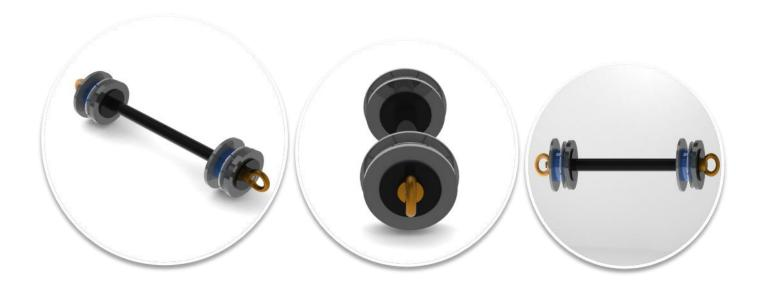
Designed to be used for riser, J-tube, spool; and another type of mechanical pull-through application. This is achieved by passing a wire through the pipe and then connecting it to the front end of the scraper which is fitted with a certified pulling point. The scraper can then be winched through the pipeline.
