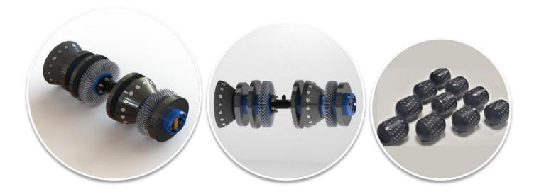
Generally, the studded or pin-wheel scraper is designed similarly to a standard mandrel scraper, but it is fitted with a heavy-duty polyurethane disc or cup embedded with threaded ferrules uniformly arranged all around its circumferential faces into which a tungsten carbide pin or ceramic ball are mounted, similarly to a foam scraper.
