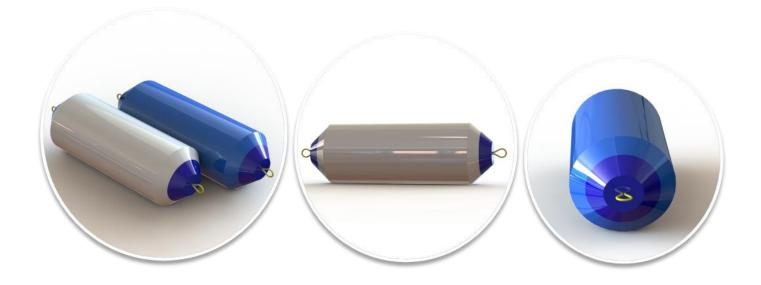
IKS manufactures marine fenders replacing standard inflatable fenders with urethanebased foam coated with a 4mm layer of high-performance PU elastomer compatible and resistant to hydrolysis and weathering harsh environments.
